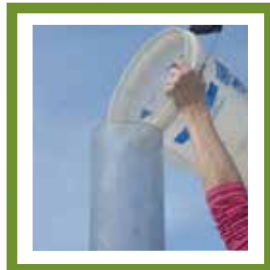
Figure 9: Filling Infiltrator with Water
