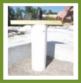
Figure 3: Hammering Pipe Into Media
